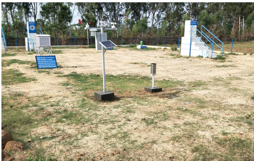
GPRS Enabled Solar Powered Telemetric Rain Gauge and Weather Station
